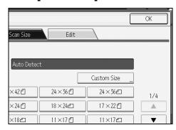
Specify Original Size (X1 and Y1) using the number keys, and then press the [#] key.
